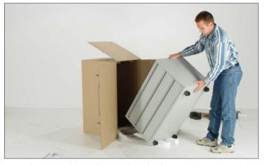
11. Bring the cabinet down using the foam strips to pivot the cabinet on. Without the foam the wheel posts could bend. The foam allows the cabinet to float above the wheels while it is angled down into the horizontal position.
