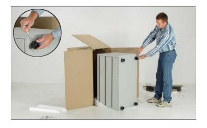
9. The locking wheels go at the front of the cabinet and the non-locking wheels at the rear. Use a ½ inch or 13 mm wrench or pliers to tighten the nut at the wheel post firmly.
