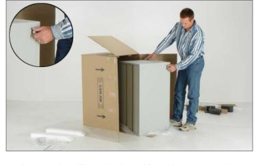
8. If you are installing wheels on this cabinet unscrew the levelers on the bottom of the cabinet. The wheels will replace those levelers.
