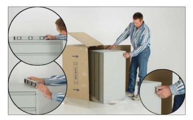
5. Check the levelers. If you are stacking this cabinet, or using a caddy, the levelers should be all the way in. If this is the base cabinet, the levelers will be used to level the cabinet. The levelers will also serve to lift the cabinet off the floor slightly. This is especially important on carpeting. You want the levelers carrying the weight - not the bottom of the cabinet. Tilt the cabinet forward and backward to access the levelers when it is in position and ready to be leveled.
