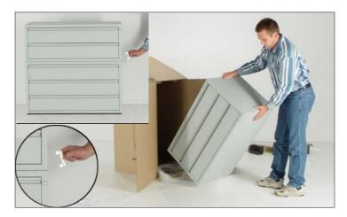
6. Set the cabinet down gently. The cabinet should be leveled precisely where it will be used. Use a level and be sure the cabinet does not wobble. If you are stacking the cabinet you **must** use the safety C-Clamps provided to join the cabinets. Slide the C-Clamp Tabs into the holes at the rear of the cabinets ensuring the tiny slats in the tabs are pointing down and forms the letter "C" from the rear when installed. Any questions? Feel free to call us during office hours EST.
